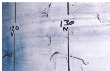
Figure 2: Surface defects related to seamless pipes [1]
